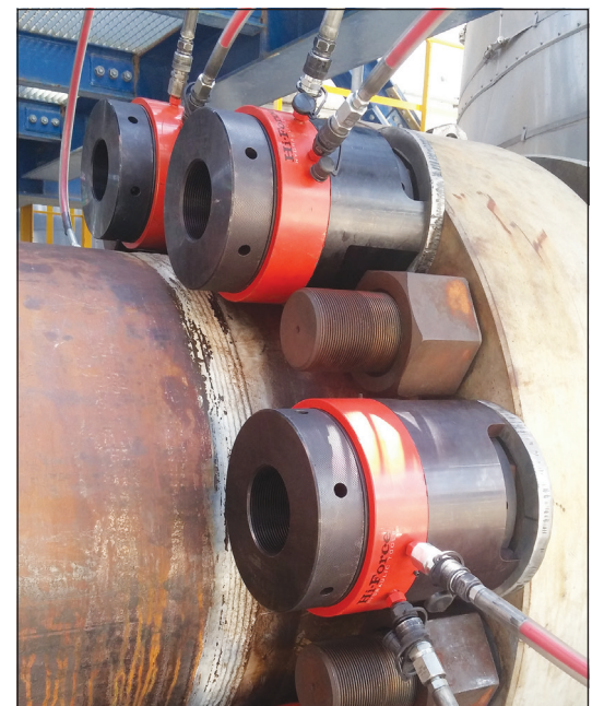
Hi-Force hydraulic bolt tensioners ... doing the job efficiently and accurately
