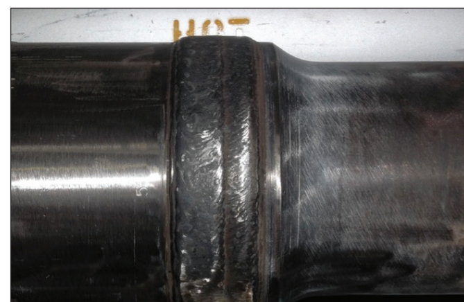
Duraband NC hardbanding applied to a Pin Tool Joint
