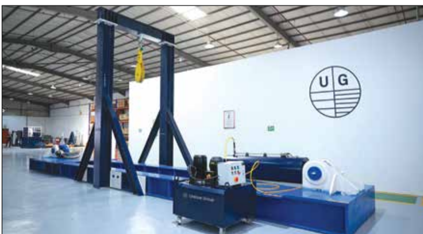
Saudi Arabia's largest dynamic winch test bed
