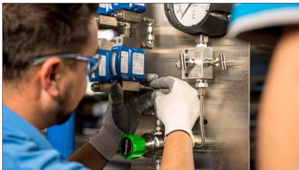
Figure 3 ... Changing seal support systems to standardised panels can make installation, service, and maintenance easier while improving component performance over their lifetime
