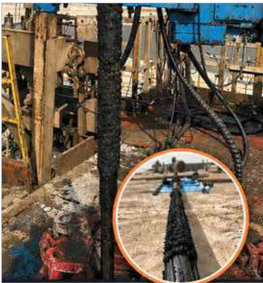
About 45 kg of metal debris was retrieved in a single bottom hole assembly run
