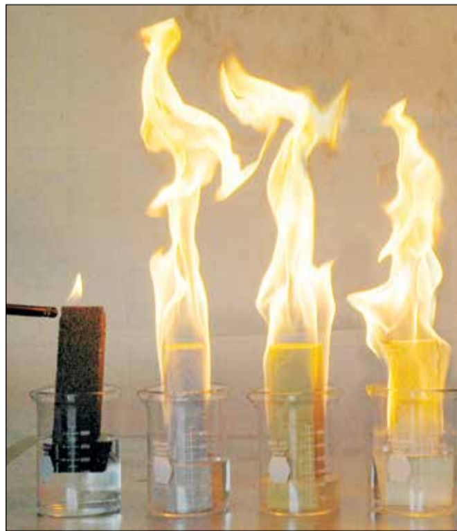
Wicking of different insulation materials after absorption of combustible liquids
