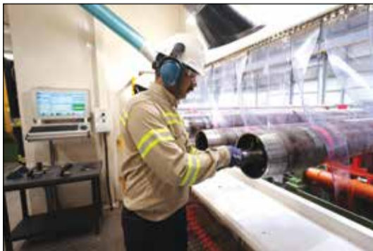
The facility is the first in the UAE to thread full-length premium connections
