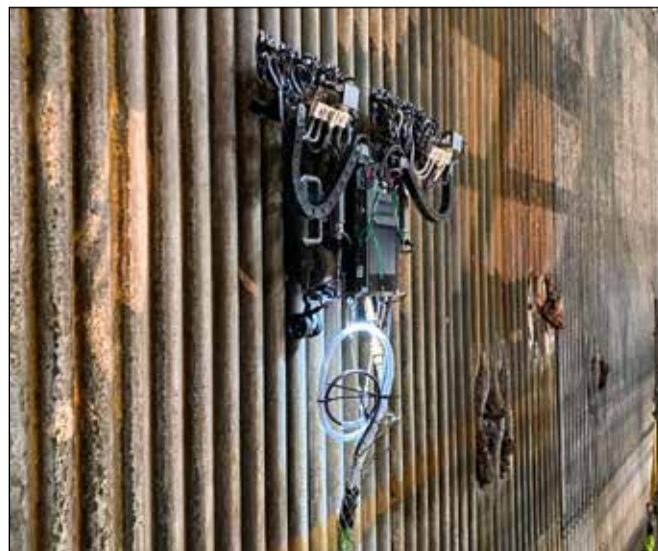
Gecko's wall-climbing robots use specially designed sensor payloads to build sophisticated digital maps of assets
