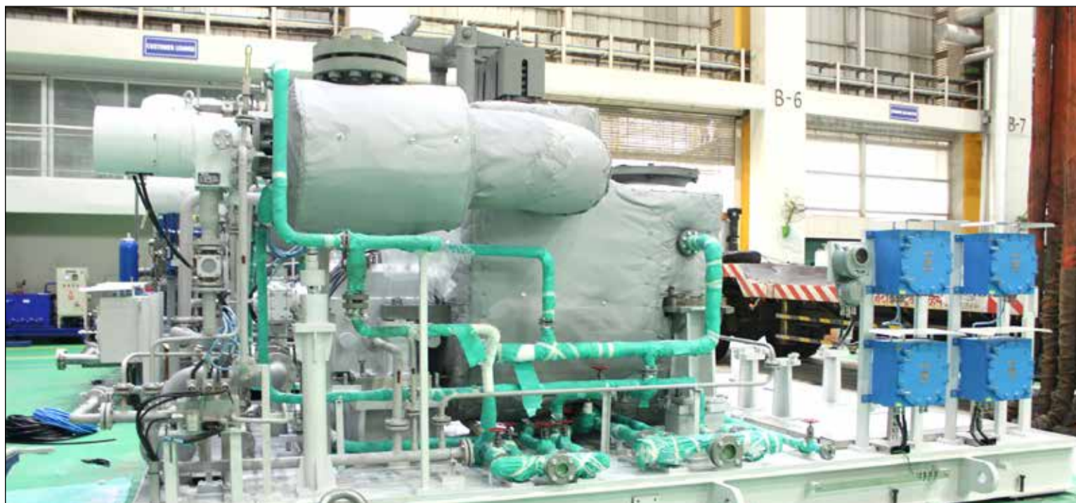
A 3.6 MW STG ready for dispatch to a client in India
