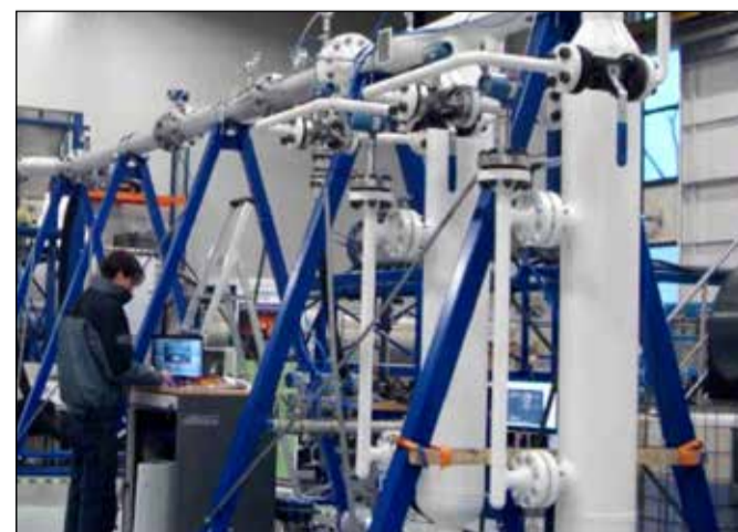
Sulzer's compact HiPer™ Deoiling Hydrocyclone skid and (right) compact HiPer™ TwinLine™ separator (inline separation)
