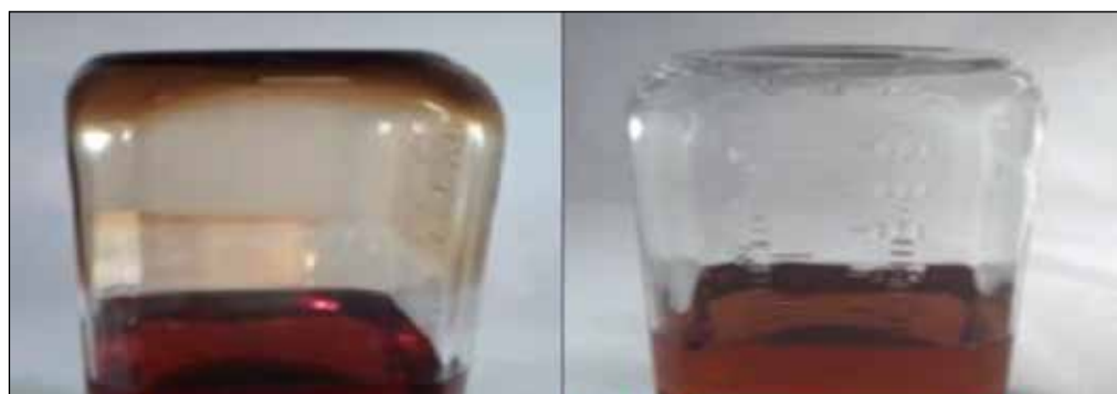
Figure 1 ... Film formation in untreated (left) versus treated (right) samples
