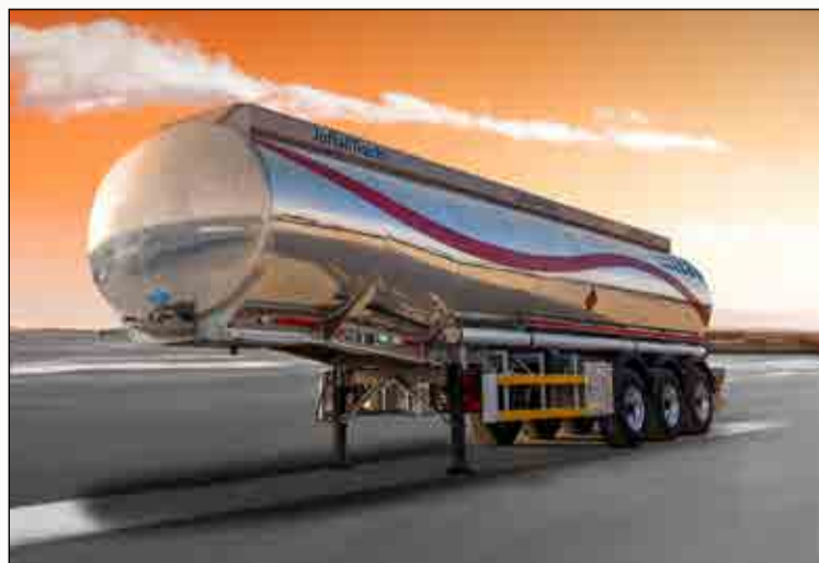
An aluminum tank trailer reduces fuel consumption for the towing vehicle
