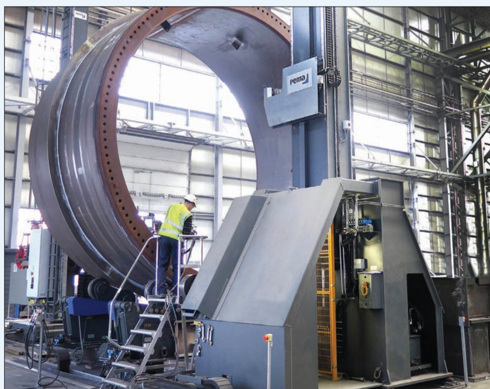
The PEMA flange fitting station for onshore and offshore wind-towers
