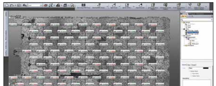
Quick detection of areas beyond tolerances ... indicated by the value and highlighted in red
