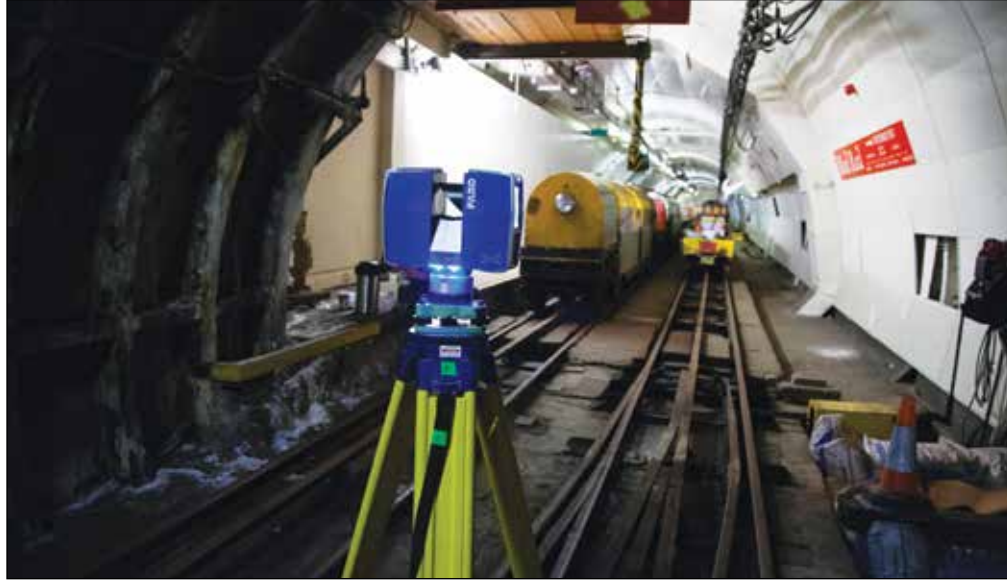
The Faro scanner can finish scanning the inner wall of the tunnel in minutes
