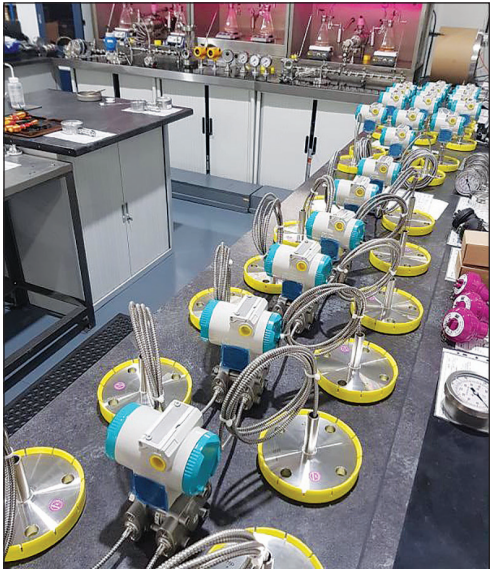
Siemens transmitters free issued to PCI by a leading distributor for the fitting of bespoke diaphragm seal systems
