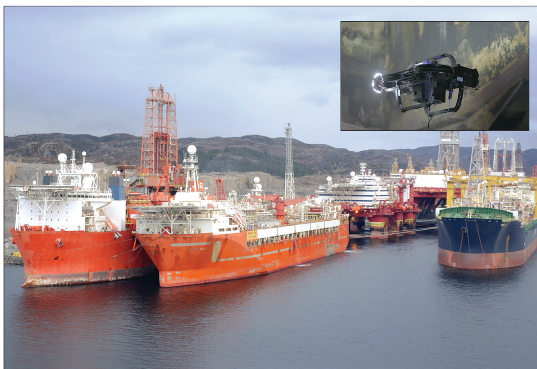
The Petrojarl Varg FPSO unit inspected using drones (inset)
