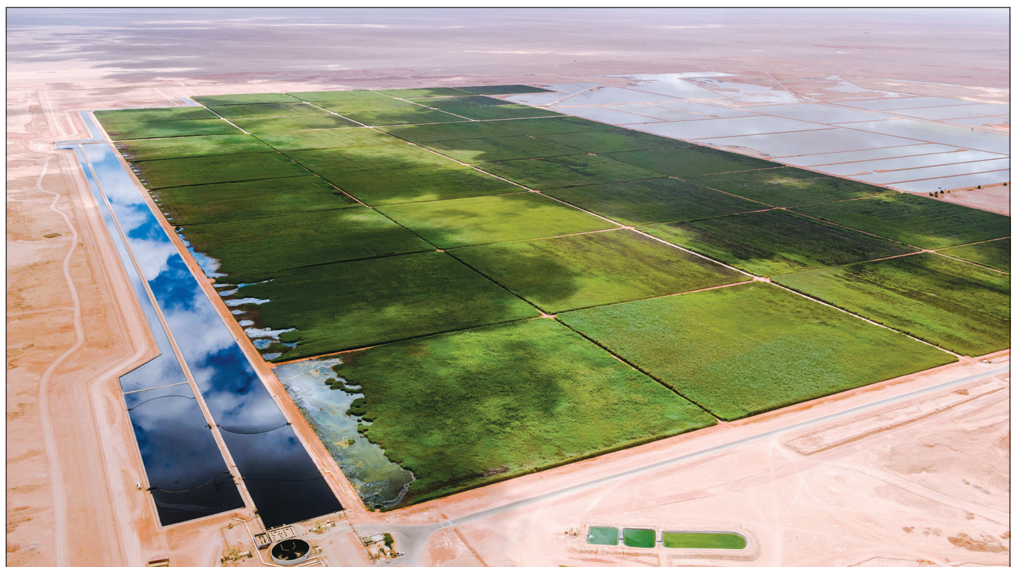
The Nimr water treatment plant processes over 110,000 cu m per day of produced water from the Nimr oilfields in the southern Oman desert
